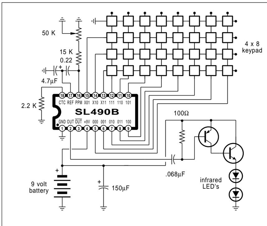
Fig. 1 – This handheld infrared remote control transmitter can send up to 32 different commands. Each command outputs a repeating code consisting of six brief pulses of infrared light.
