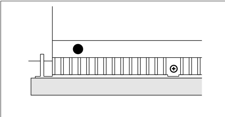
Fig. 2 – Continue modifying your CX cartridge by drilling this 1/4 inch hole in the spent toner holding tank underneath the cartridge. When you are done reloading, seal up both holes with a very aggressive tape. Be sure to replace the cardboard label and the fuser wiper pad after refilling. Finally, do a light dusting of the drum with *Pixie Dust* or another drum conditioner.
