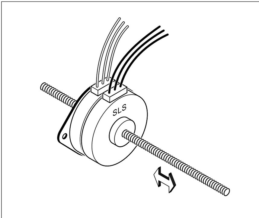
Fig. 3 – THIS HURST SLS LINEAR ACTUATOR is a real "sleeper" for new hardware hacking. This easy-to-drive 12 volt, 12 watt unit offers 24 pounds of force in two mil increments. Use them in pairs for X-Y motions. What can you do with these that are new and unique?
