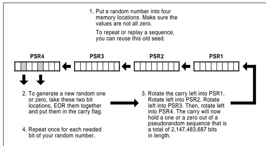
Fig. 3 – A 31 stage pseudorandom sequence generator done in software will produce a "random" string of 2,147,483,687 ones or zeros before it will start to exactly repeat. Typical execution time is under 40 microseconds.
