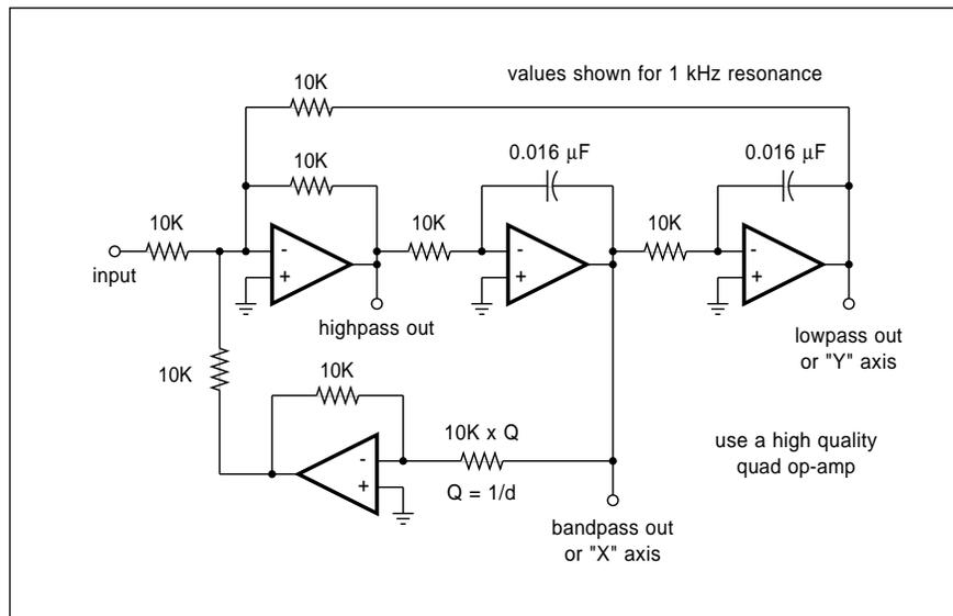
Fig. 4 – THIS STATE VARIABLE ACTIVE FILTER can give you lowpass, bandpass and highpass outputs, and is a good "workhorse" circuit for both low and high Q uses. This is also a handy test circuit for exploring phase plane plots on your own.
