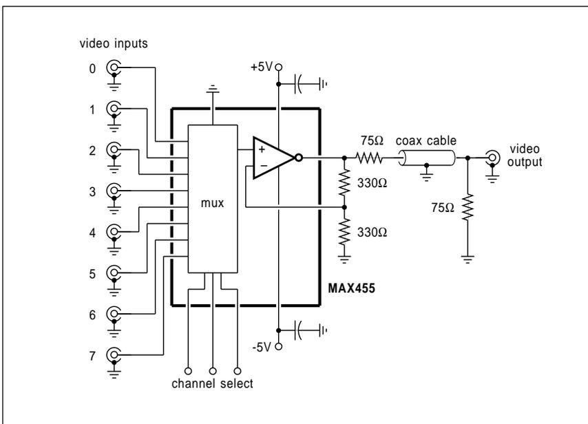
Fig. 3 – An eight position, single chip video selector and driver.
