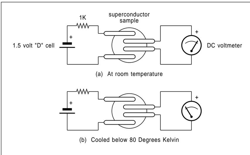
Fig. 1 – A test circuit to demonstrate the zero internal resistance properties of a cooled superconductor. The meter will show you zero voltage when your superconductor is below its critical temperature. The "four point" measuring scheme is used to minimize the effects of contact and lead resistance.
