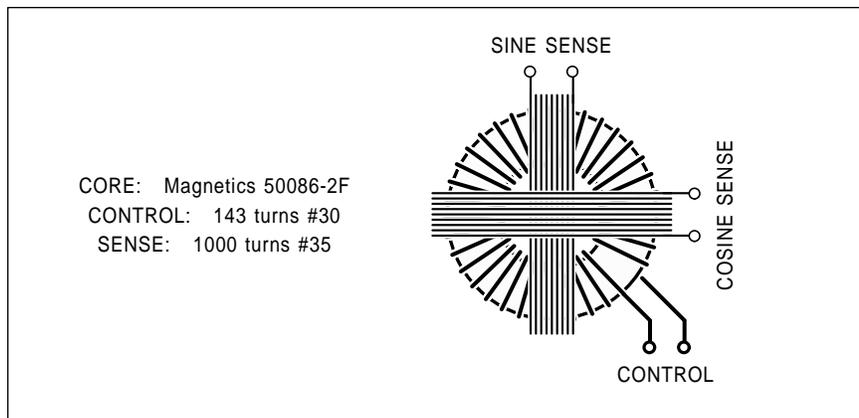
Fig. 3 – Adding a new quadrature sense winding will give you both the sine and cosine of the field strength. When one is weak, the other will be strong. The tangent of the final magnetic bearing is found by dividing the sine output by the cosine output. A list of possible winding details are also shown.
