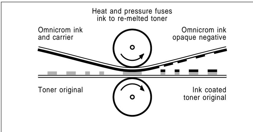
Fig. 1 - The Omnicrom process rapidly converts any toner based copier or laser printer image into full color in any of dozens of metallic, matte, or special effect shades. Kroy Sign Systems now licenses the British Omnicrom process under the US tradename of Kroy Kolor.
