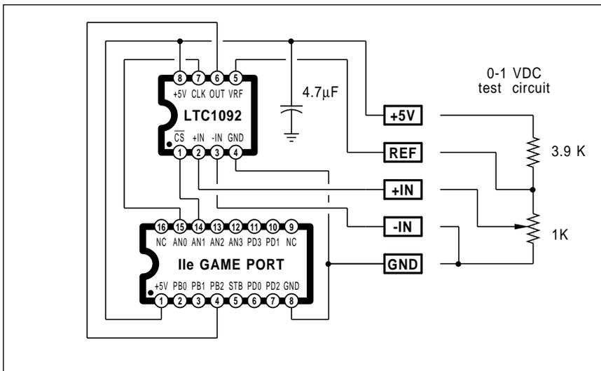
Fig. 3 – This 10-bit floating point a/d converter is very easy to interface to an Apple IIe, IIgs, or most any other personal computer or microprocessor.
