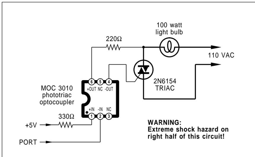
Fig. 1 - This ac power output interface lets you directly control 100 watt lamps and other high power loads from your microcontroller or your personal computer. The special phototriac optocoupler provides safety isolation. Note that a low logic input will light the lamp.
