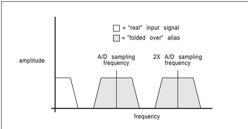
Fig. 2 – An anti-aliasing filter absolutely must be used with any A/D converter so as to sharply reject any and all frequencies above one-half of the sampling frequency. Should any higher frequencies remain present, they will "fold over" and form aliases that end up looking just like "real" input signals.
