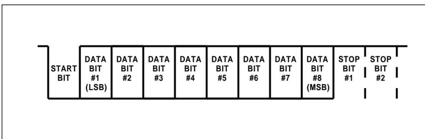
Fig. 3 – Most RS-232 serial communications will use this older "teletype" asynchronous code. Seven or eight data bits are normally used, with the least significant bit always sent first. Any number of stop bits above the minimum can be sent between successive characters.
