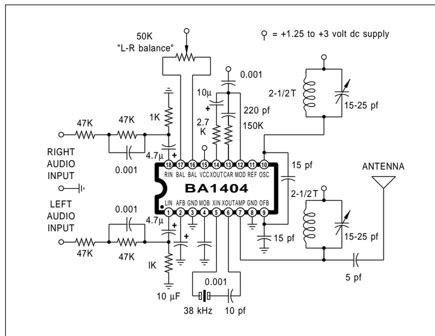
Fig. 4 – A MICROPOWER STEREO FM wireless broadcaster that is low in cost, works off one AA cell, uses few parts, and offers high audio quality.
