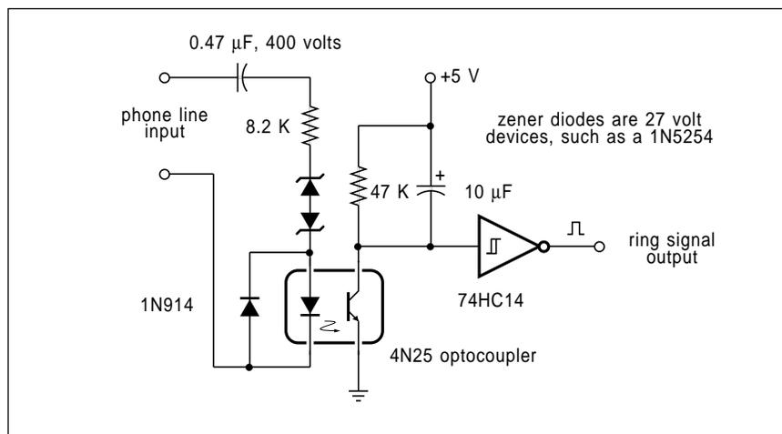
Fig. 4 – A telephone ring detector. The optocoupler provides safety isolation, while the capacitor converts the individual rings into a continuous signal.
