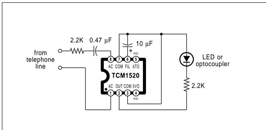
Fig. 4 – This telephone ring detector might be used to light a LED or to power a LED optocoupler to create an isolated "the phone is ringing" digital signal.
