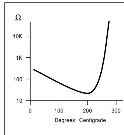
Fig. 1 – A typical resistance versus temperature curve for a posistor. If you exceed the critical temperature, the resistance sharply increases and the current dramatically drops.
