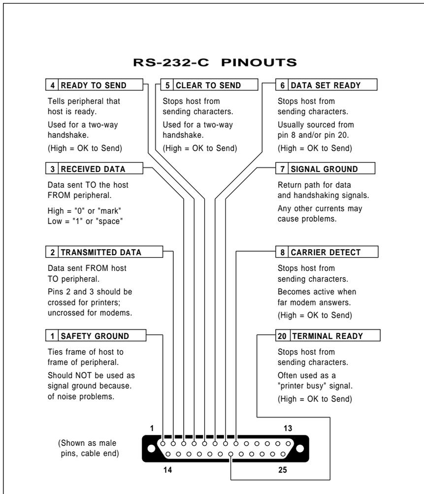
Fig. 1 – Here are some details on the RS-232 serial communications standard. Note that the data and handshake lines are often crossed for printers and uncrossed for modems.
