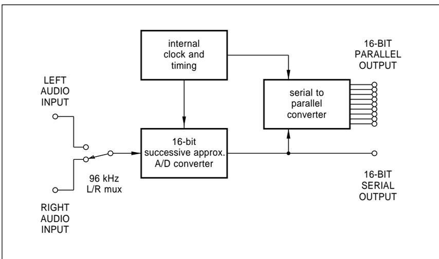
Fig. 2 – A SIMPLIFIED BLOCK DIAGRAM of the CDB5126 stereo audio A/D front end board. Because of a factory tested layout, nearly all of the usual black magic involving ground noise, shielding, and guarding has been done for you.
