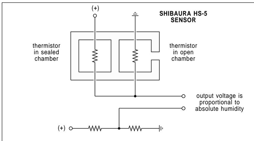
Fig. 4 – THIS NEW ABSOLUTE HUMIDITY SENSOR from Shibaura uses the difference in the thermal conductivity between dry and humid air to produce an output voltage. Both thermistors are run in their self-heating range.
