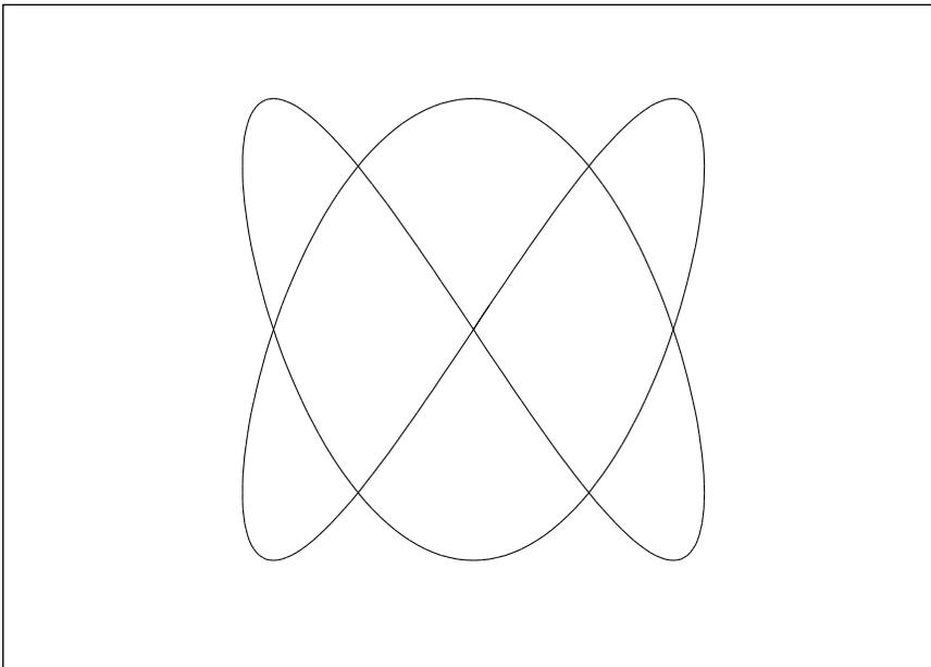
Fig. 6 – The Lissajous figure is the oldest of phase plane plots. The two sinewave frequencies shown here are in a ratio of 3:2.
