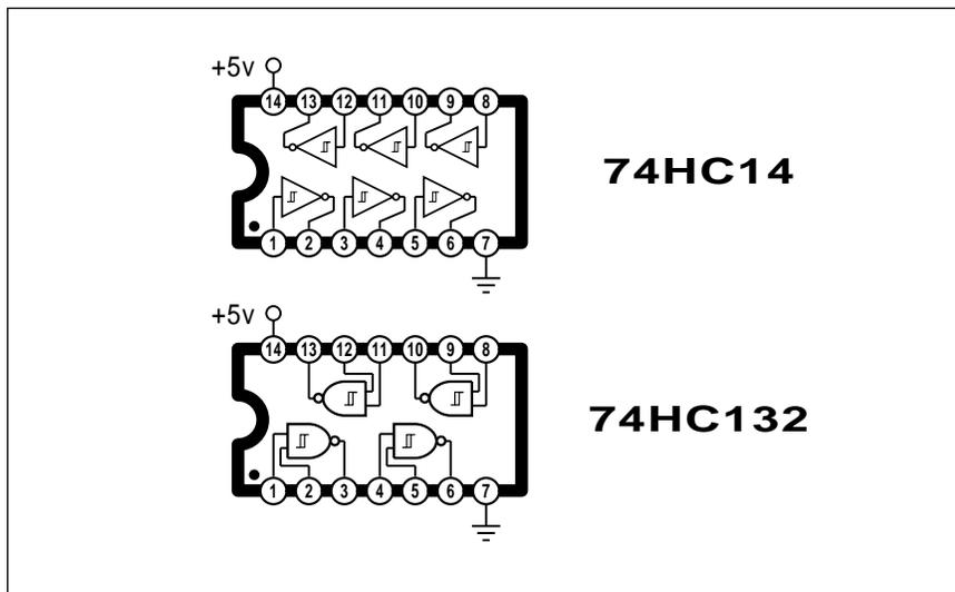
Fig. 2 – THE PINOUTS FOR THE TWO most popular CMOS Schmitt chips include both the hex inverting 74HC14 and the quad NAND 74HC132. While intended for +5 volt use, they will work over a +2 to +6 volt range. For higher voltages, use the older 4093 or 4584 devices instead. Note that both of the chips are shown top view.
