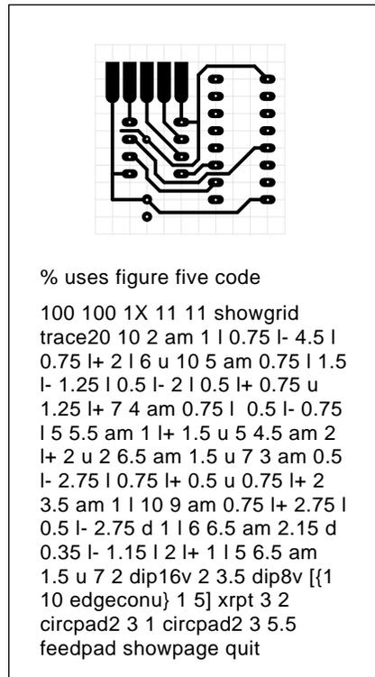
Fig. 6 – TYPICAL PC LAYOUT. Omit the *showgrid* command to delete the fine gray viewing grid.
