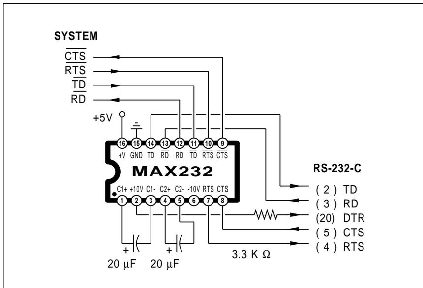
Fig. 4 – This RS-232 driver circuit needs only a single +5 volt supply. An internal charge pump circuit generates the needed +10 and -10 volts for the actual interface levels.
