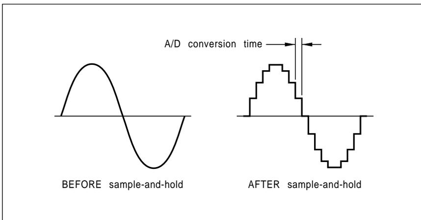
Fig. 3 – A sample and hold is needed to hold the analog input signal constant during the conversion time, or serious errors are certain to result.
