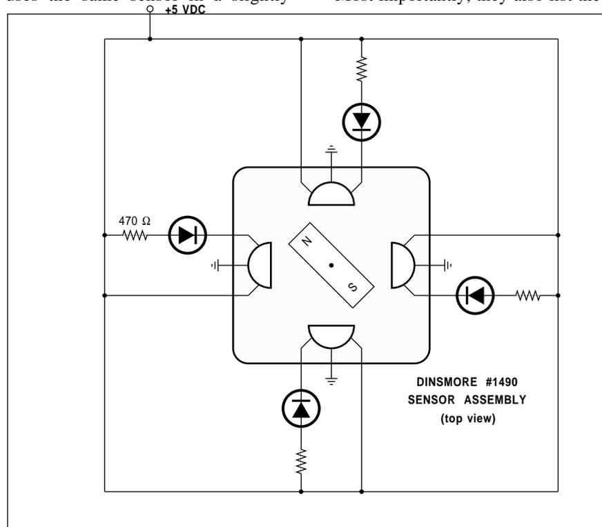
Fig. 5 – LOW END DIGITAL COMPASS is cheaper than a fluxgate but has a very poor resolution. Hall effect sensors are used to drive the LED outputs as shown here. Eight point LCD compass rose displays are also possible.
