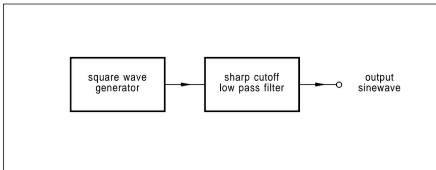
Fig. 1 – Brute force generation of a digital sinewave creates a square wave and then sharply low pass filters it. Triangular or certain "magic" waveforms can give you much better results than a square wave.
