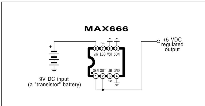
Fig. 5 – This linear regulator drops down a 9 volt battery to give you a fixed +5 volt output at up to 40 milliamperes. The standby current is a mere five microamperes.
