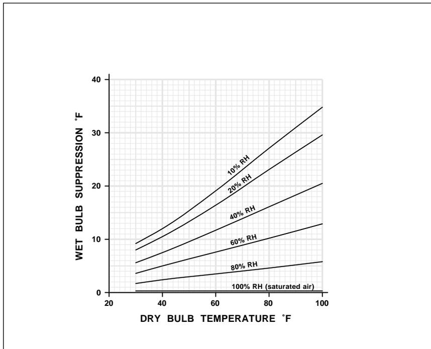
Fig. 2 – WEATHER FORECASTERS OFTEN will use a wet-bulb, dry-bulb sling psychrometer to measure the relative humidity. The lower the humidity, the more the evaporative cooling of the wet bulb, and the lower its temperature. This graph calculates the relative humidity for you.
