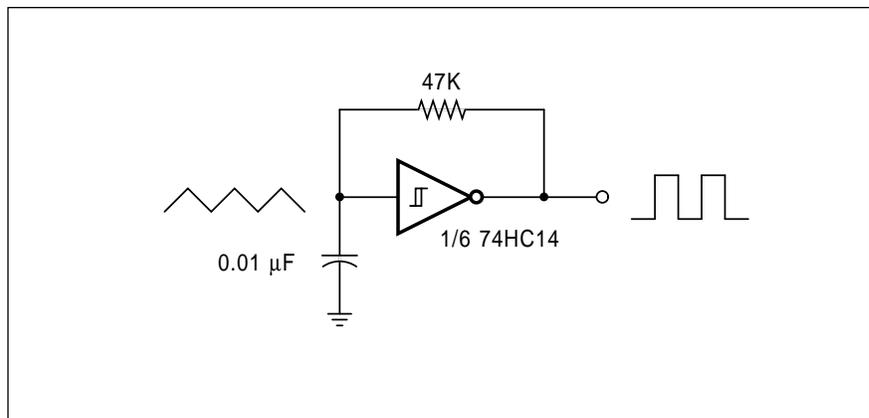
Fig. 1 - AN ELEGANTLY SIMPLE oscillator can be built using nothing but one resistor, a capacitor, and 1/6th of a CMOS hex Schmitt Trigger. Your output is a full supply square wave, while the input is a triangular wave that "saws" between the trigger's upper and lower trip points.
