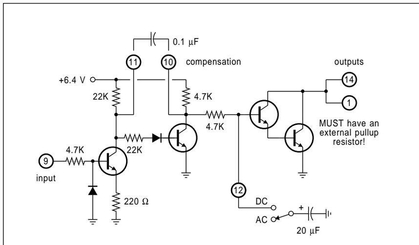
Fig. 5 – The ULN 2429 detector turns on with a square wave input greater than 1.2 volts peak-to-peak, and stays off otherwise. The filter capacitor can select either an AC or a DC output.
