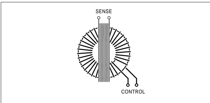
Fig. 2 – A fluxgate magnetometer is built by using a control winding that is able to alternately saturate and unsaturate its toroidal core. When the earth's magnetic field does get sucked into and out of the core, it will induce pulses into the sense winding. All these induced pulses are proportional to the strength and the direction of the field.
