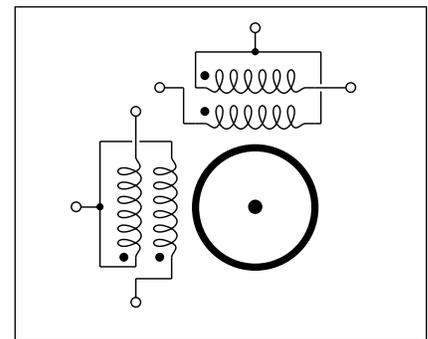
Fig. 2 – IN A UNIPOLAR (or bifilar) stepper motor, you will find a pair of windings for each phase. While this raises the cost and also reduces the available stepper power, your driver circuitry is vastly simpler and very much cheaper, since only a current sink is needed for each winding. A unipolar stepper often has six leads.
