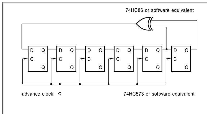
Fig. 1 - A six stage pseudorandom sequence generator gives you 63 six-bit binary numbers in an apparently random, yet exactly repeating order.
