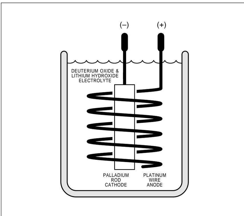
Fig. 4 – COLD FUSION appears to get produced in this experimental electrolytic cell. The heavy water dissociates into deuterium and oxygen ions. The deuterium ions will migrate to the palladium cathode where many of them become trapped in its crystalline structure. Some of the later arriving deuterium ions apparently cold fuse with the trapped ones, apparently producing both heat and at least a few of the expected fusion by-products. But it is far too soon to tell for sure.
