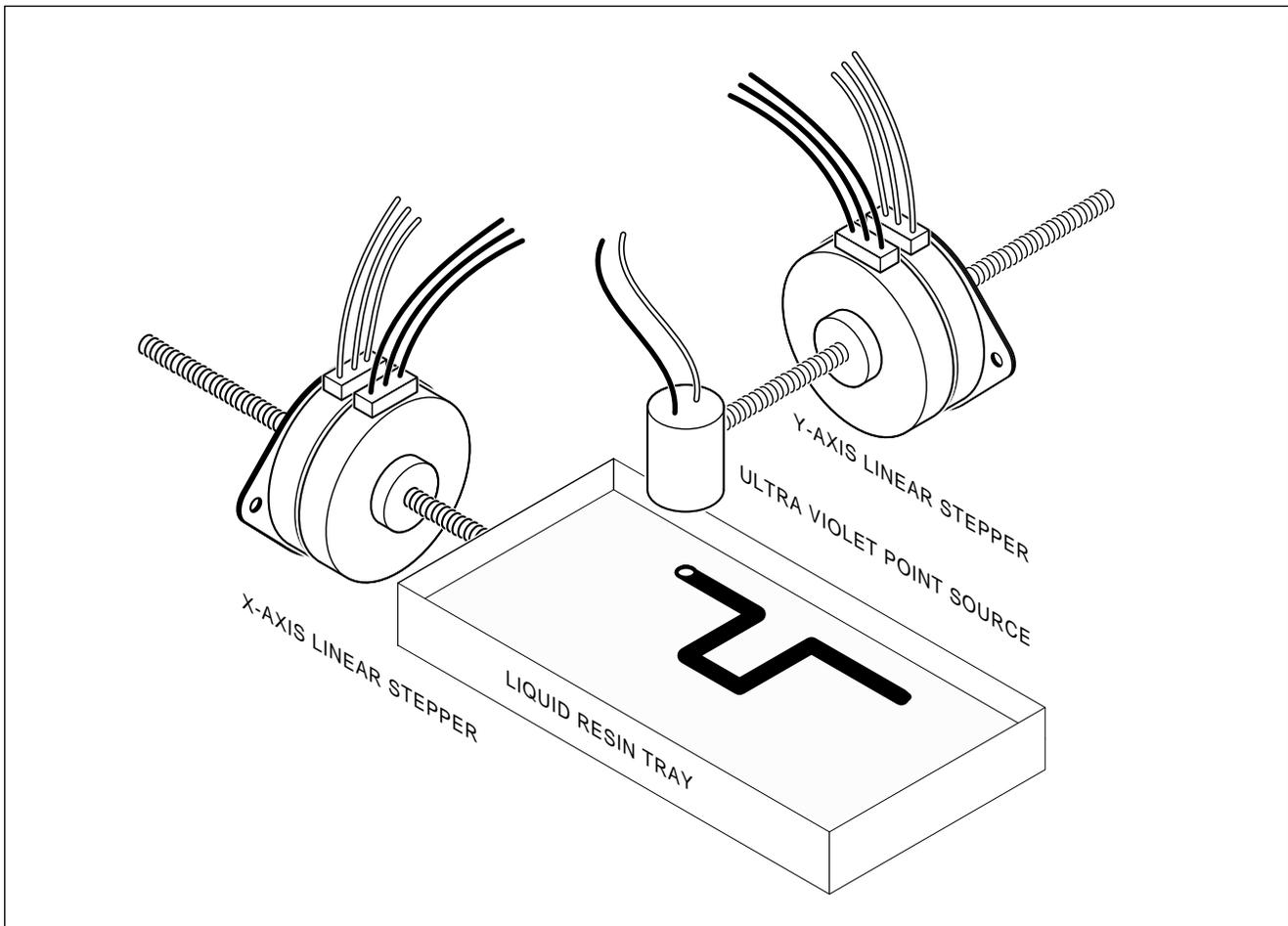
Fig. 4 – A two-dimensional santa claus machine can create a replica of virtually any flat object through the selective ultra-violet hardening of a liquid plastic photopolymer resin. Any object can be created anywhere in the world.
