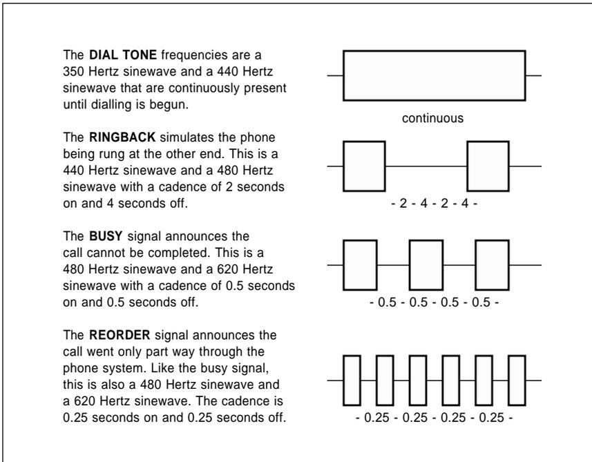
Fig. 1 – TELEPHONE CALL PROGRESS signals can be detected by both their frequency and their cadence. Here are all the US standards for the "precise" or the "new" call progress tones.
