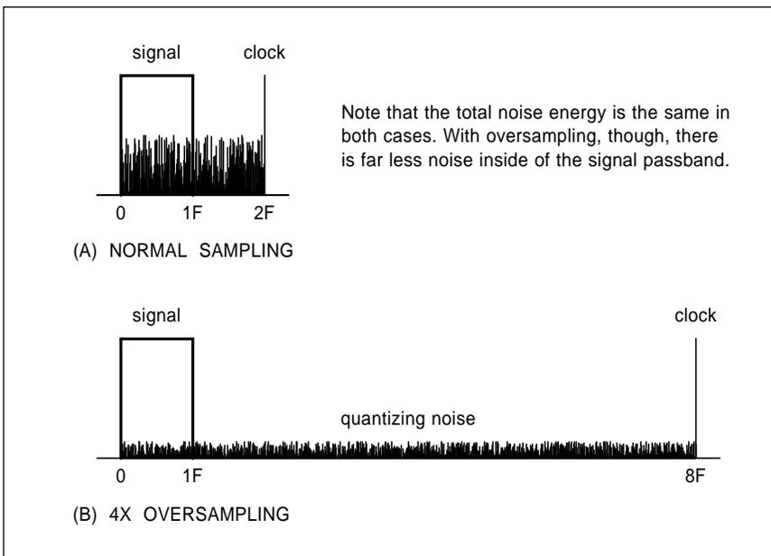
Fig. 5 – THE QUANTIZATION NOISE of an A/D converter is often distributed from DC on up to the sampling frequency. By oversampling and then digital low pass filtering, a 1-bit A/D converter can actually end up with far less noise than a 16-bit one! This is one of the key secrets to Crystal's Delta-Sigma conversion and post decimation digital filtering scheme.
