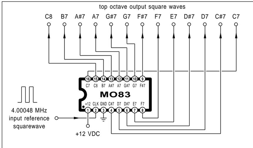
Fig. 5 – A top octave generator integrated circuit takes an input reference square wave and divides it down to approximate the thirteen uppermost notes on an electronic organ. Further binary division of each output can generate all the needed lower notes. This SGS part replaces the Mostek MK5083.
