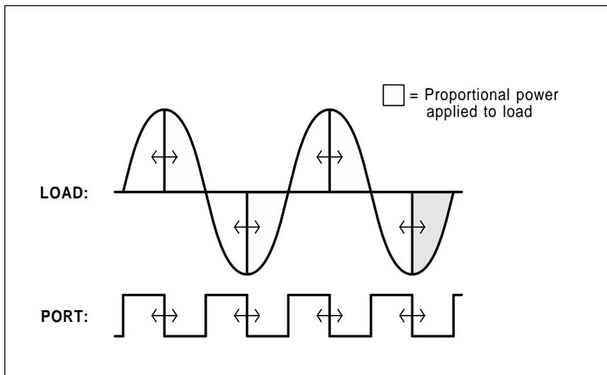
Fig. 3 – The secret to brightness control is to use a duty cycle or a "phase" modulation. Apply power early in each half cycle for maximum brightness; later for less. Use incandescent lamps only.
