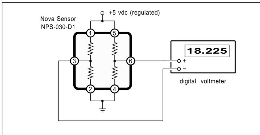
Fig. 4 – This simple circuit will get you started experimenting with the new solid state pressure transducers. This sensor is rated at a relative 0-5 PSI.
