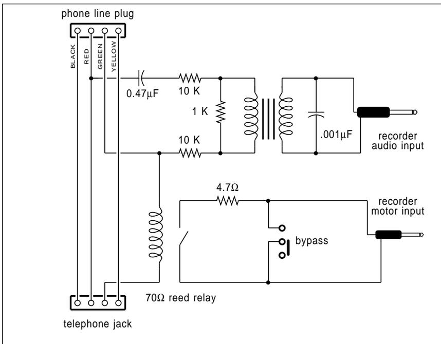
Fig. 3 – An audio access arrangement can record both sides of a telephone conversation, but is only legal for use under certain circumstances.
