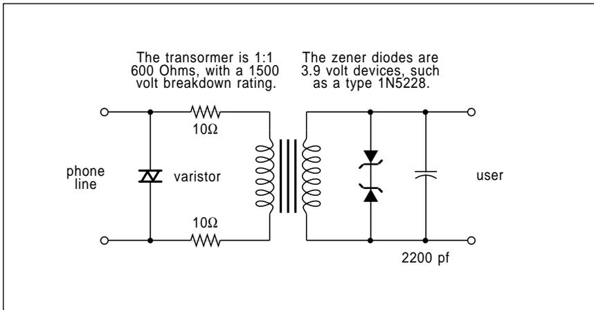
Fig. 2 – A data access arrangement such as this one must provide for surge suppression, signal limiting and safety isolation, as well as being FCC part 68 type approved.
