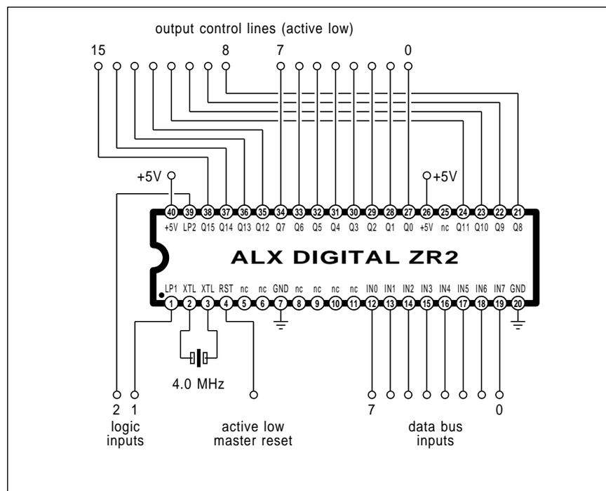
Fig. 5 – THE ZR2 "DISCO CHIP" is programmable to handle many light chasers, zoners, and ac/dc dimmers, along with other communications, counting, and control tasks. It is based on a programmable peripheral interface chip from Intel.
