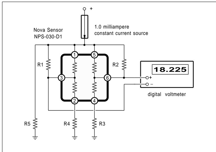
Fig. 5 – Extra resistors can be provided for temperature compensation and for span adjustments. Correct values are specified for each sensor.
