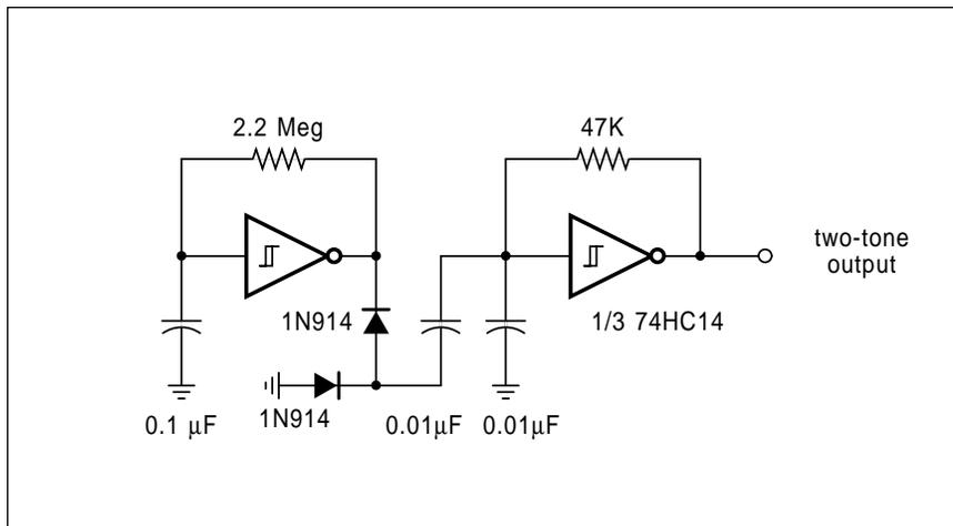
Fig. 4 – THIS TWO-TONE ALARM produces a distinctive "twee-dell" output. The spread between the high and low pitch is set by the ratio of the two right timing capacitors. Experiment to get the best-sounding results.
